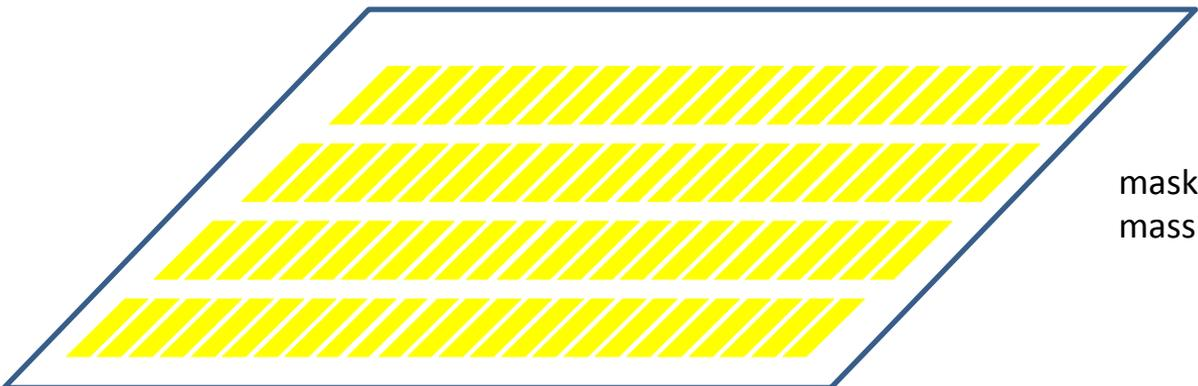
mask removed and sample analyzed in MALDI mass spectrometer
